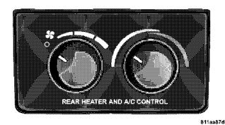
The rear compartment control uses two rotary knobs: one for the temperature control and the other for the fan speed control. The mode for the rear air conditioning and heating system is always controlled by the front control unit. Fan and temperature can be controlled from the front control unit or the rear control unit.
